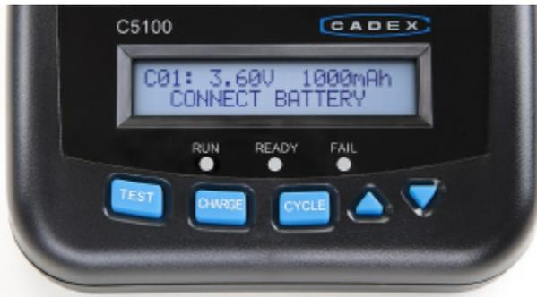
**TEST:** Sorts Li-ion into *Good*, *Low* and *Poor*.
